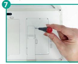
Lock the screw into the screw hole.
