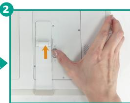
Slide the latch to unlock the SSD door.
