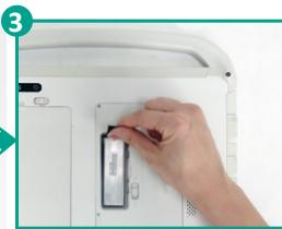
Pull the tape on the top of the SSD door to loosen the SSD.
